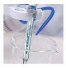
3. Take the electrode out of the solution and rinse it with distilled or deionized water.\*
