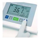
3. Press the calibration button on the pH meter and wait until the measurement is stable.
