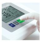
2. Press the measurement button on the pH meter and wait until a stable endpoint has been reached.
