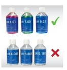
Select the correct buffer group or buffer values for the calibration in the meter's settings.
