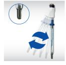
3. Check the tip of the electrode for air bubbles. If found, shake the electrode like a thermometer.
