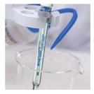
4. Take the electrode out of the solution and rinse it with distilled or deionized water.
