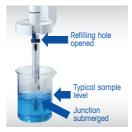
2. Pour enough pH calibration buffer into a measuring beaker and dip the pH electrode into the first buffer.
