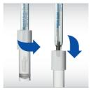
2. Remove the wetting cap from the pH electrode.
