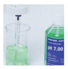
1. Place the electrode in a beaker with reference electrolyte solution or pH buffers 7.00 or 4.01.
