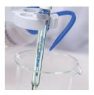
6. Rinse the electrode with distilled or deionized water.
