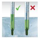
5. For refillable electrodes only: check the electrolyte level (artificially colored green for illustration purposes) and refill if necessary.
