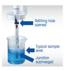
1. Pour enough sample solution into a measuring beaker and dip the pH electrode into the sample.
